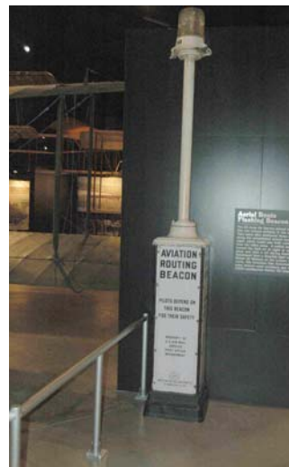
The system used 284 beacons approximately 10 miles apart. A sequence of Morse letters identified the beacon in each segment: WUVHRKDBGM which pilots remembered using the sentence " When Undertaking Very Hard Routes Keep Directions By Good Methods. "
