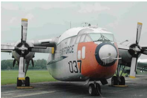
The aircraft pictured above is the actual plane which recovered Discoverer 14. Note the direction finding antennae on the nose which were used to "bird dog" the descending parachuted payload.
