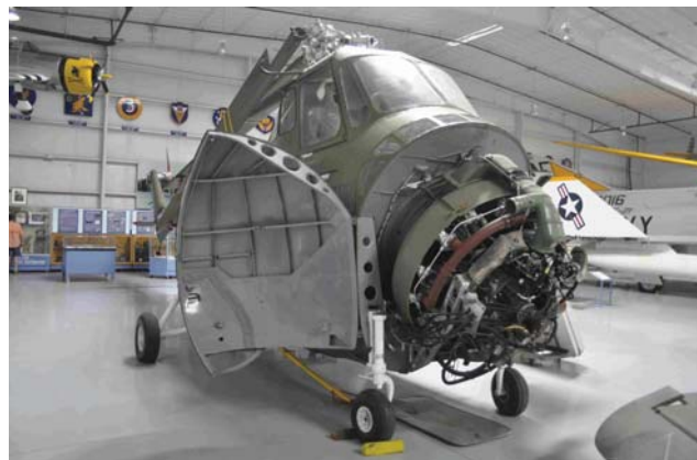
The Sikorsky Model 55, US military H-19 Chickasaw displays the unusual mounting of its radial power plant which could be changed in two hours.
