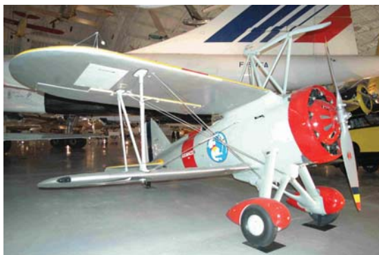
Note the Trapeze Hook Mounted on this Sparrowhawk carrying U.S.S Macon Identification
