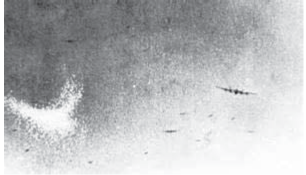
RAF photo of an Avro Lancaster deploying chaff, the v-shaped “cloud” on the left side of the frame. (Photo Credit: RAF)
