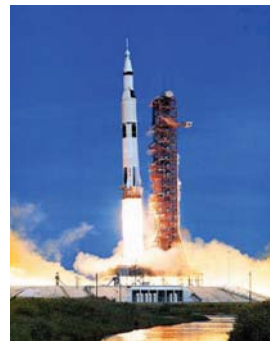
Apollo 15 at launch. 6.2 million pounds of weight powered by 7.6 million pounds of thrust. (Photo Credit: NASA)
