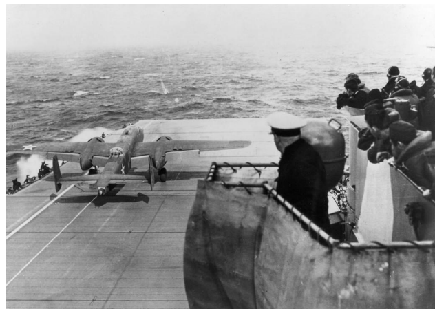
B-25 departing. The combined wind speed and ship speed gave a wind across the decks of 50 knots. Lift-off speed was 68 knots with full flaps and full rear stick.
