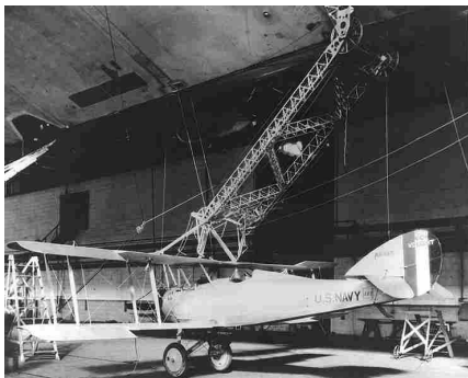
The trapeze used to hook the aircraft was developed. However, the Los Angeles had no hangar and the aircraft could not be brought aboard. Her successors would be so equipped.
