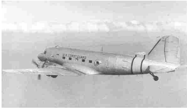
A R4D carries the wide yellow band just forward of the empennage marking it as an air-sea rescue craft.
