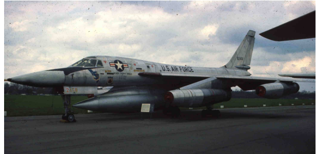
"Area ruled" Convair B-58 Hustler, first USAF supersonic bomber and winner of the 1962 Bendix Transcontinental Air Race.
