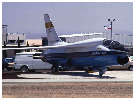
Vought TF-8A Crusader modified with a supercritical airfoil and on display at NASA's Dryden Flight Research Center.
