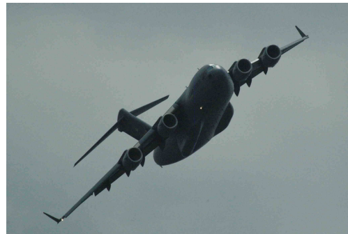
Winglets on a McDonnell-Douglas C-17 Globemaster III.
