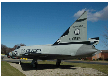
Convair F-102 first to take advantage of the "Area Rule," and flown by the 103rd Fighter Interceptor Group out of Bradley from 1956 to 1971
