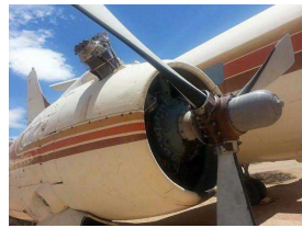
The top of a piston and a blown jug
