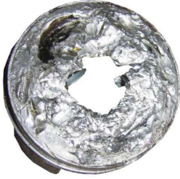
The top of a piston and a blown jug
