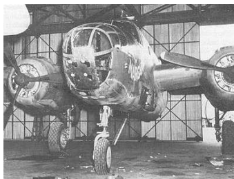
Right: Quad .50 caliber guns in B-25 glazed nose and port side "cheek" guns.
