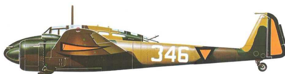
This P&W Twin Wasp Junior engined Fokker G.I (so-called 'G.Ib') was one of those ordered by Spain but confiscated by the Dutch on 10 May 1940. Hurriedly painted in LVA Markings and given the number 346 it was assigned to 4 JaVa, but on 13 May had brake failure and was captured intact by the Luftwaffe.
