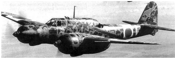
Note the Japanese version of Schräge Musik. The angle is 30 degrees which differs from the Luftwaffe's 60 degree arrangement.
