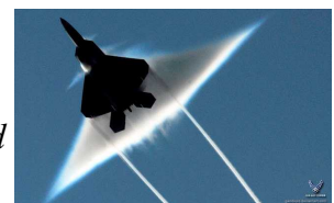
“Indie” wields his whip and a conical shock wave is delineated by the condensation of air caused by the drop in pressure behind the F-22.
