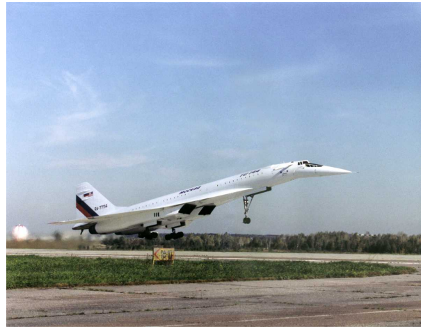
Dryden Flight Research Center EC98-44749-19 Photographed SEP1998 The Tupolev Tu-144LL Flying Laboratory lifts off the runway at Russia's Zhukovsky Air Development Center near Moscow on a high-speed research flight. (NASA photo by Jim Ross)
