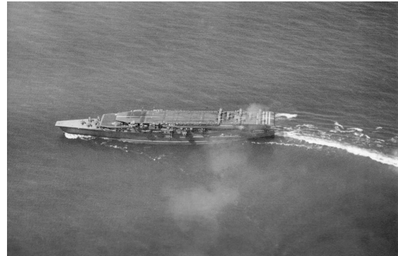
Note the triple flight deck of the Kaga. Mitsubishi B1M bombers are on the top deck and Nakajima A1N fighters are parked forward on the lower deck.
