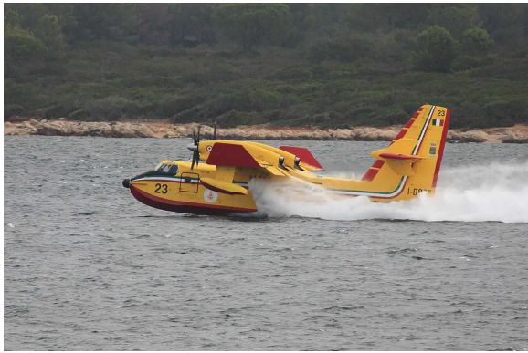
This Italian based Bombardier CL-415, on the step, in the act of scooping up water. (Credit: Horticultural marxist)
