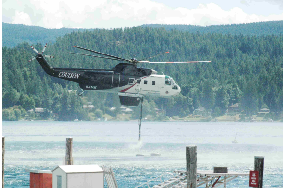
One of Coulson's S-61s Uses a a Snorkel to Fills it Belly Tank at Sproat Lake, British Columbia.
