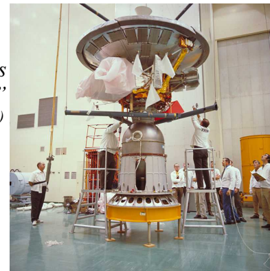
Pioneer Ten Mounted on its “Kick Motor.” (Credit: NASA Ames)
