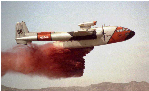
A Fairchild C-119 Packet equipped with an dorsal mounted auxiliary turbojet. (Credit: Steve Whitby)
