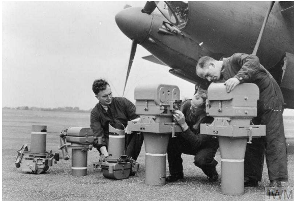
(left to right) two F.24 14-inch lens vertical cameras, one F.24 14-inch lens oblique camera, two F.52 vertical cameras with 20-inch lenses (Credit: Imperial War Museum)
