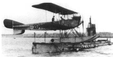
The 24 foot long aircraft perched on the 20 foot beam of the U-12.
