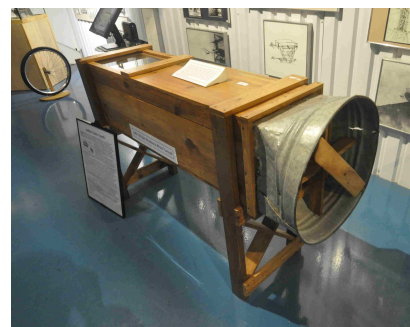
Above, a bicycle modified with a force balance and used by the Wrights to test airfoils, a converse wind tunnel. Below: A replica of a Wright wind tunnel on display at the General Thomas Stafford Aerospace Museum.
