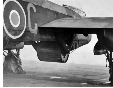
The cradle and bomb were mounted externally.
