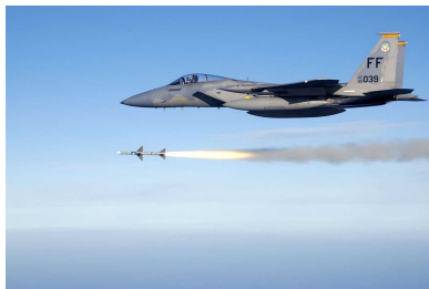
Fox One is the NATO call announcing the launch of a semi-active radar homing missile.
