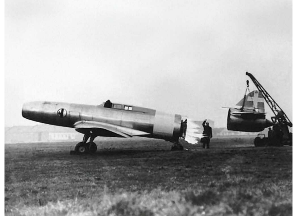
The N.1 tail has been removed to study the combustion.
