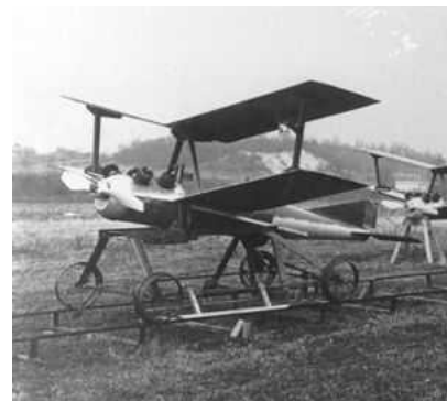
A launching system using a rail and a falling counterweight as devised by Orville Wright to accelerate the Bug to flying speed.
