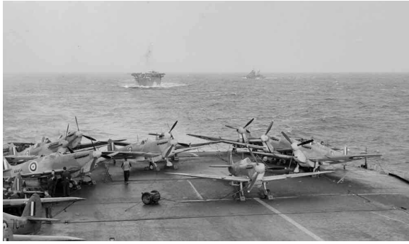
The graceful lines of the Spits are marred by the Volkes air filters needed to protect the engines on dusty Malta and the belly mounted 90 gallon slipper tanks to extend their range.
