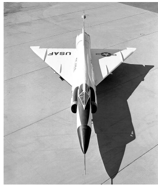
The YF-102, a subsonic aircraft had the area rule applied and it became the Mach 1.5 F-102A.
