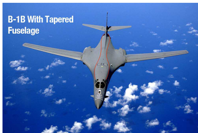
The constant cross-section design allows the Bone to reach Mach 1.25 at altitude.
