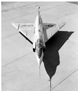
The YF-102, a subsonic aircraft had the area rule applied and it became the Mach 1.5 F-102A.
