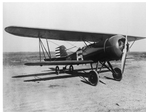
Curtiss AT-5A Hawk with a NACA cowling which added 19mph to its speed.
