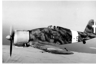
The Fiat G.50 Freccia (Arrow) was slow, short ranged, had a limited endurance and suffered from an open cockpit.
