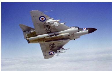
FAW.9R carrying four de Havilland Firestreak air-to-air heat seeking missiles.
