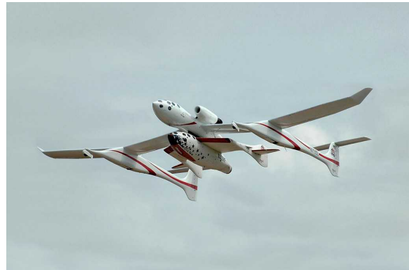
White Knight and SpaceShipOne. Note the similarities of the forward portion of each aircraft. White Knight also served as a flight trainer for the SpaceShipOne crew.
